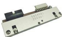
CA/ THERMAL PRINthead
